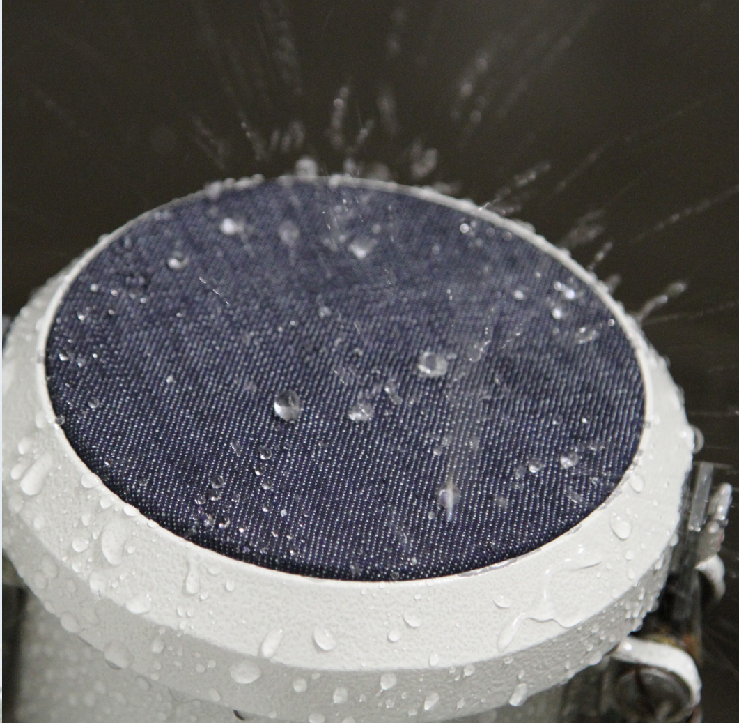
Bundesmann test for the evaluation of water repellency carried out at RUDOLF GROUP.
