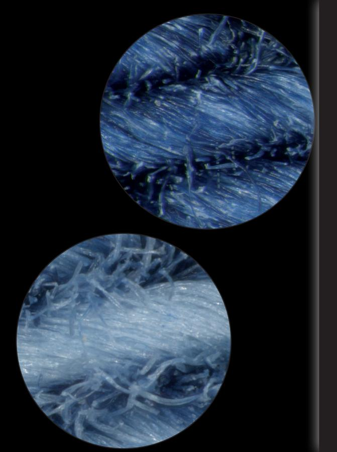
**Above**: denim untreated, lasered and washed. Result is a standard laser abrasion.
